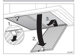
■ To remove the grease filter pull the locking clips forward, lower the filter down 45°, unhook it at the rear, and take it out.
